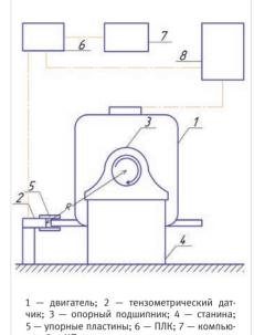
1 - motor: 2 - tenzometric sensor: 3 - support bearing; 4 - frame; 5 - thrust plates; 6 - PLC; 7 – computer; 8 – VFD
